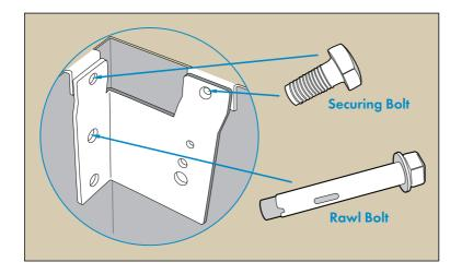
3 Position outer frame over pit, bedding on sand and cement, ensuring spring brackets are in contact with the vertical pit wall.
