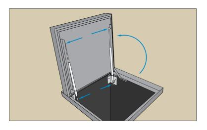
5 Open cover using Lifting Bar, attach Gas Springs as marked on spring.
