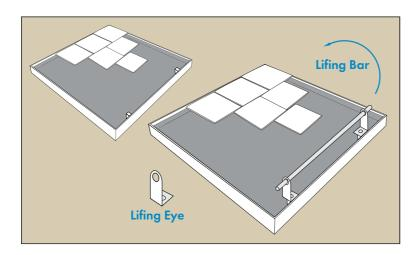
4 Close cover placing spacers between the cover and outer frame prior to filling and tiling.
