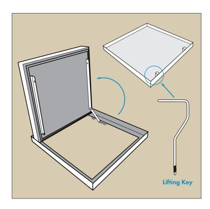
Remove cover securing bolt and open cover using Lifting Key.
